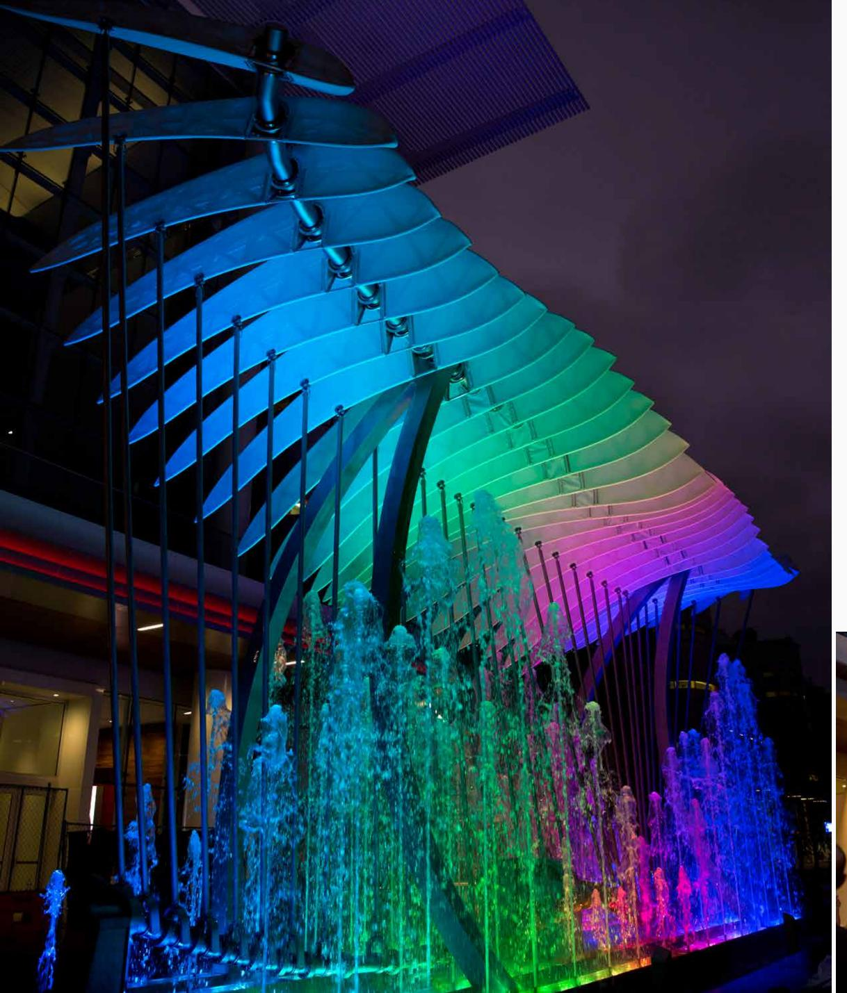
A massive yet ethereal wing, supported by two arcing supports, undulates above as an intricate mechanism rotates below. The 32 individual curvilinear organic wing elements ripple from the center out, actuated by linear pushrods driven by the turning of a helical shaft. The entire artwork stands in a pool among carefully controlled water jets and is illuminated from below with carefully controlled colorful patterns.
